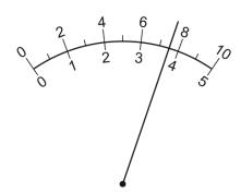
Which current is the ammeter measuring?
