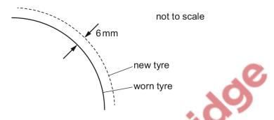
What is the error in the speed shown on the speedometer after this wear has taken place?
